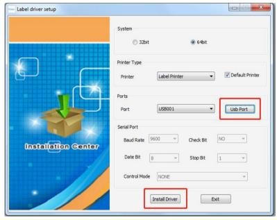
If it pop up error message "no usb printer", it's probably because the printer is not connected to computer correctly. Please double check if the printer is switched on(blue light on top is on) and connected to computer via the black USB cord, or switch to another usb port on the computer to try.
