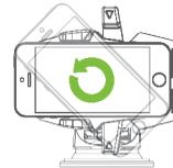
9. Adjust cradle in any angle with ball pivot joint.
