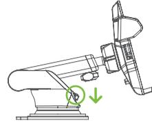
3. Pull down the lever to secure the mount.
