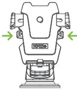
4. Press side buttons into locking position.
