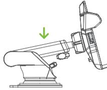
2. Unpeel sticky gel pad cover, place onto dashboard cover and press down
