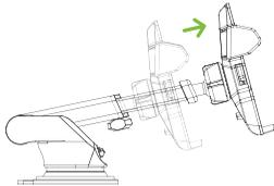
7. Loosen knob to extend telescopic arm to desired length.
