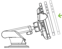
5. Place your device inside the mount firmly to activate the one touch locking system.
