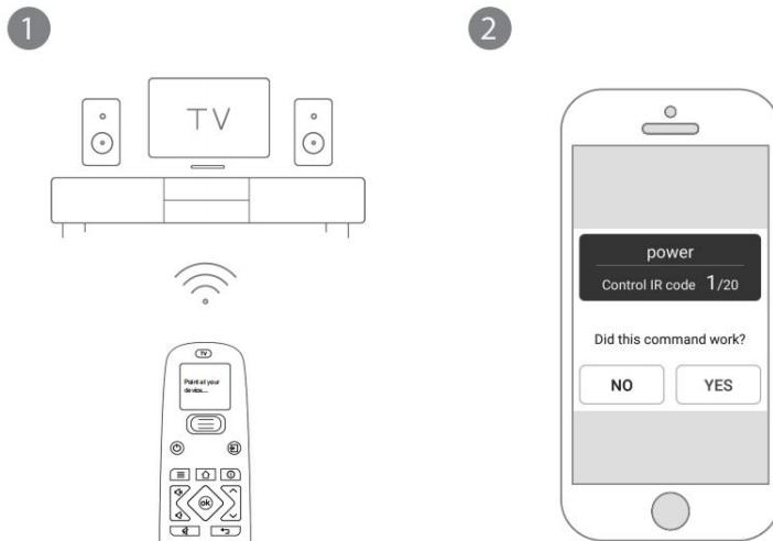
Keep your U2 in line of sight with the device. Press the first button and then choose (Yes) or (No) to see if it works. During the process, the U2 remote control will emit infrared signals to the device. U2 will be able to find the correct code set after searching the database.
