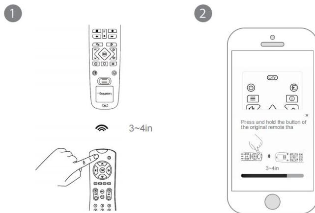
Keep your U2 in line of sight with the original remote. Select the icon of the function key you want to copy. Meanwhile, long-press the corresponding function key on the original remote.
