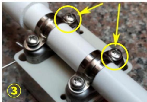
3.The pre-amplifier box is installed and fixed, tighten the four screws.
