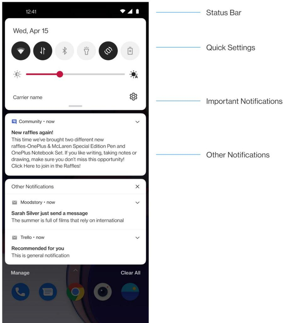
When a new system notification or app notification is received, the status bar will display the corresponding icon. Pull down the notification panel by swiping down from the top of the application page or anywhere on the home screen.
