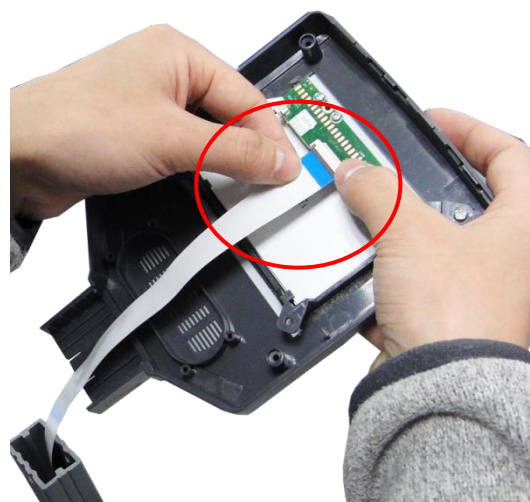
8. Open the FFC socket lock, plug and lock the FFC cable. (Note: Keep blue side upper).
