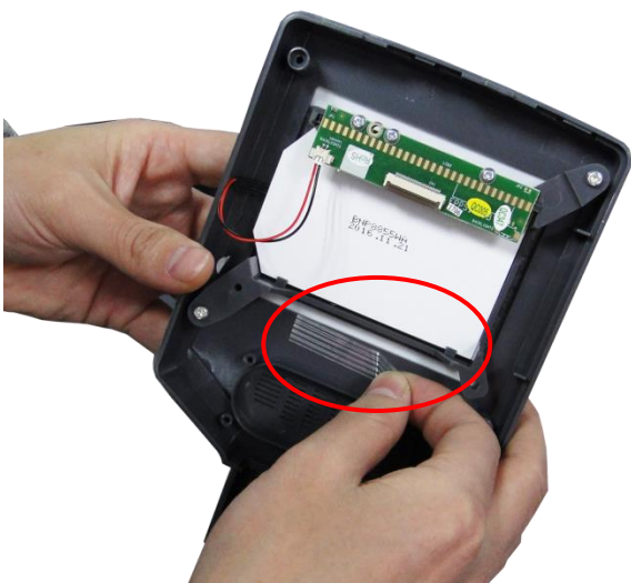
7. Remove the tape circled in the picture and stick it aside.
