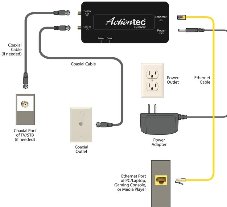
The device connected to the *Ethernet* port is now connected to the Internet via the coaxial network. Repeat this process to install additional Adapters throughout the home.
