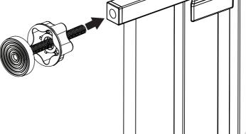
**NOTE:** The ends of the gate frame are not threaded. The *threaded spindle rods* should slide into the end of the frame tubes without any resistance.
