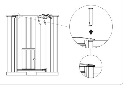
**NOTE:** Once the *spring loaded mounting pin* is inserted into the *gate door* hole, it cannot be taken out again by hand.
