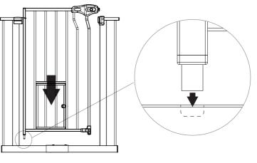
Align the hole in the upper corner of the *gate door* with the hole in the *door mounting bracket*. Insert the *spring loaded mounting pin* into the hole in the *mounting bracket* and the *door*.
