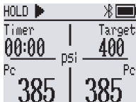
Figure 2 Enter the holding pressure test interface
