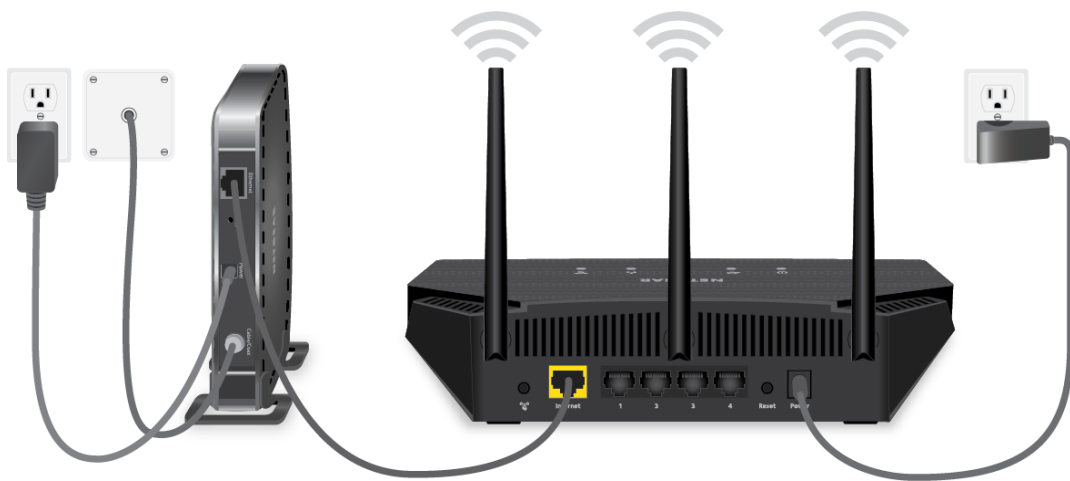
Figure 6. Cable your router
