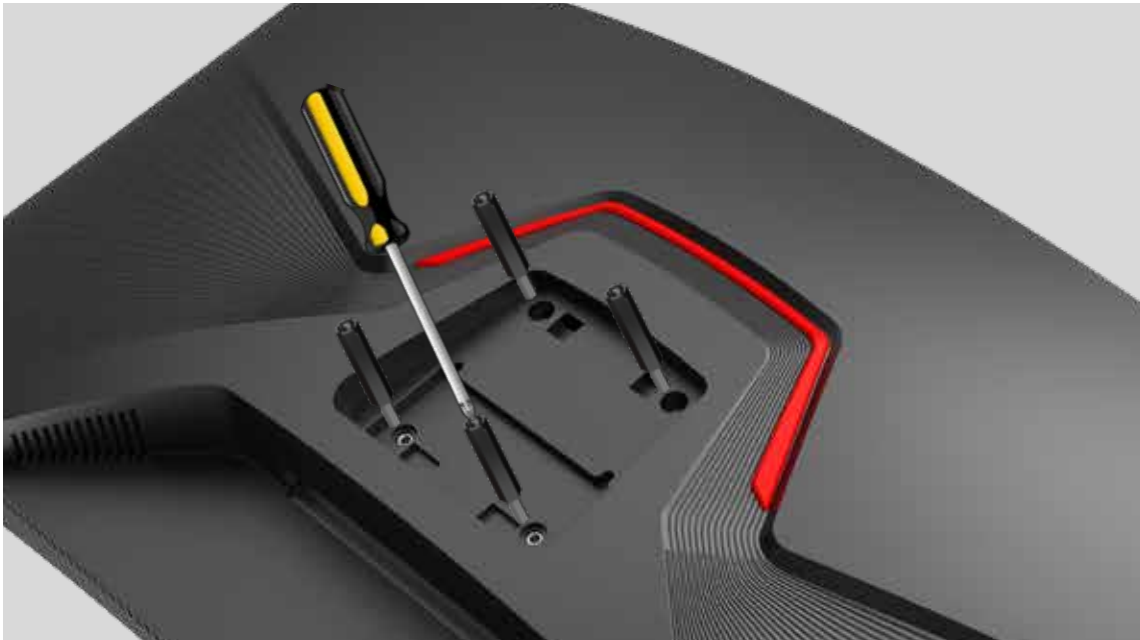
Mount the screw post or use the VESA plastic post (length not less than 24 mm).
