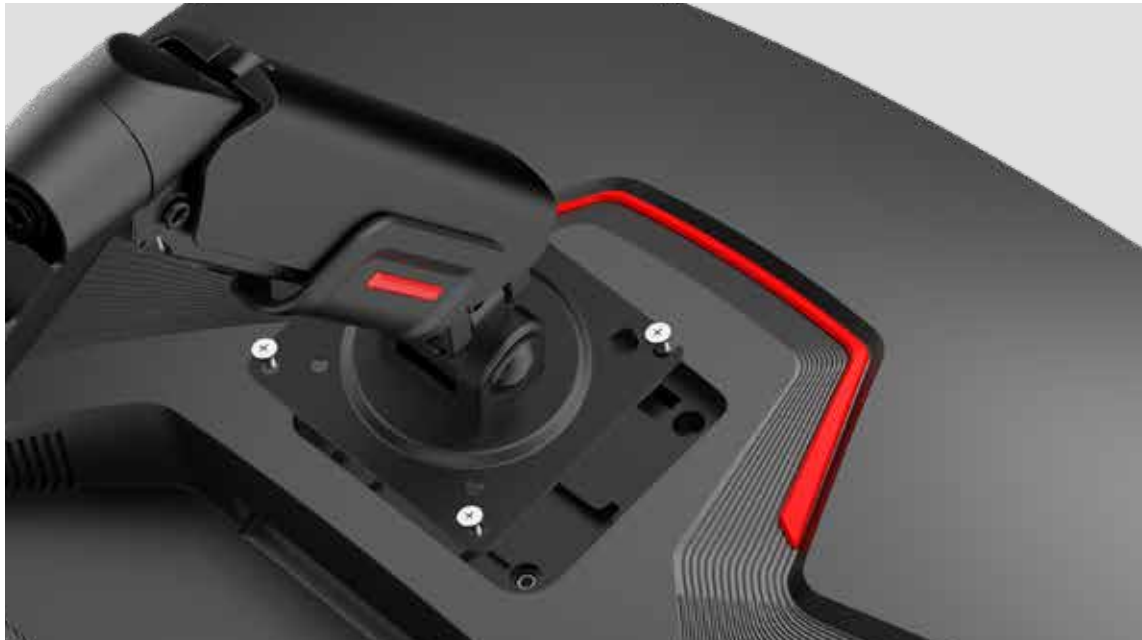
Installation screws (use screw posts, please use the rear shell screws removed in 2.2.2.1;The thread length of the locked screw is 6-8mm if the screw post is not used)
