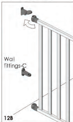
Wall fittings - B side
