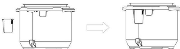
To install the condensation collector, slide it into the slot on the cooker housing. Follow the reverse order to remove it for cleaning.
