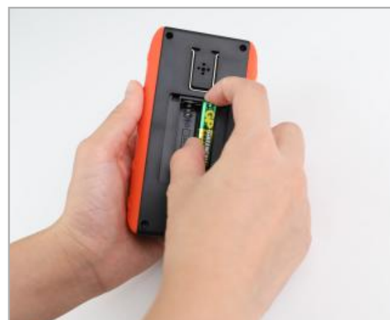
Install the batteries
