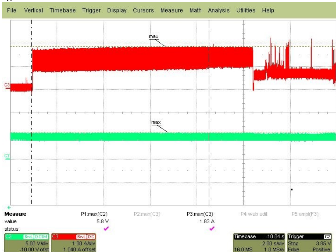
Figure 1 Typical Current Profile (5V & 12V)
