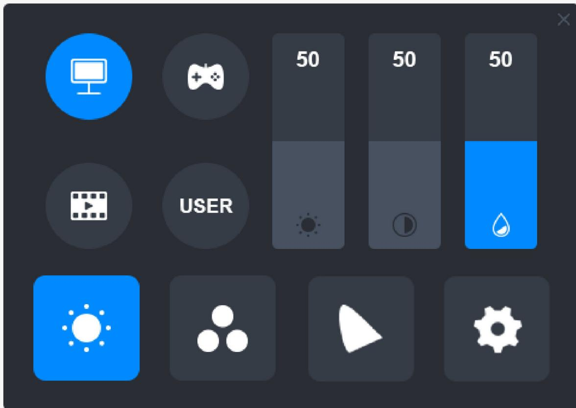
When "USER" mode is chosen, all three bars will be blue and users can adjust the brightness, contrast, and saturation by dragging them.
