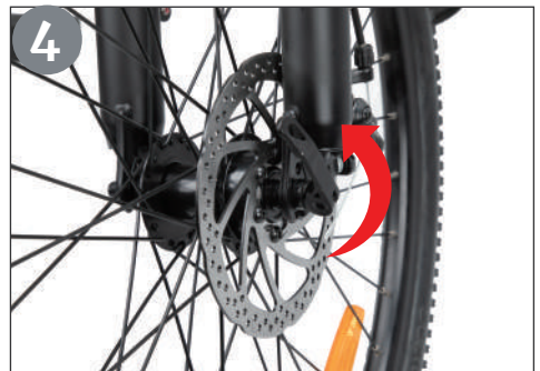
Twist the wrench upward check the operation of the wheel.
