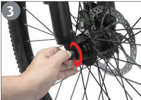
Install the quick release and then tighten well.
