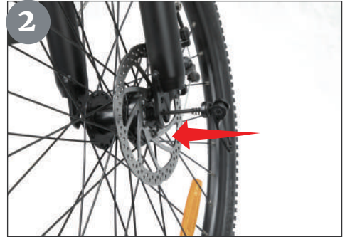
The front fork is aligned to both ends of the bearing. The disc brake is on the left.
