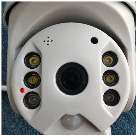
At first the indicator is **red**, and the camera is connecting to cellular network. Make sure the paring place has **good 4G signals**.
