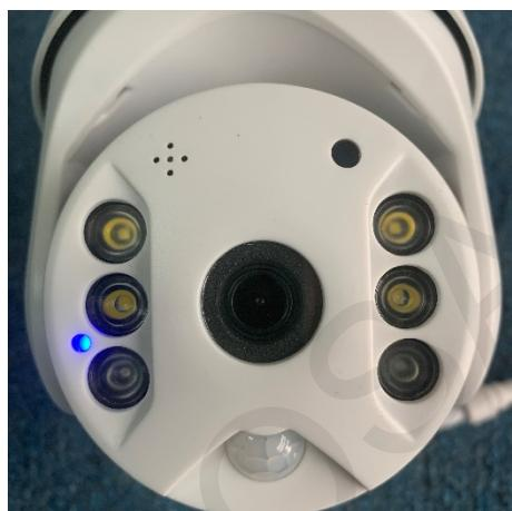
Indicator is “Blue” when it is connected to network.
