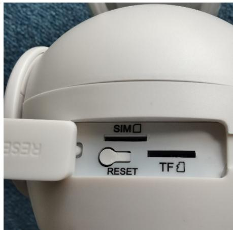
Open the silicon cap and insert the activated sim card and Micro SD card.
