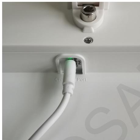
The **green light** flashes while in charging, and remains on when it is fully charged.
