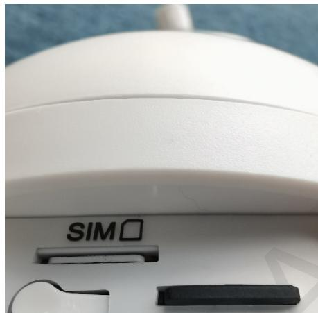
When the sim card and Micro SD card is well inserted, it should be like the picture shows.
