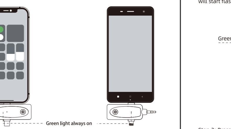
Step 1: Insert the 3.5mm receiver into the corresponding port of the device, then press the power button on the receiver. Once done, the green light will start flashing.
