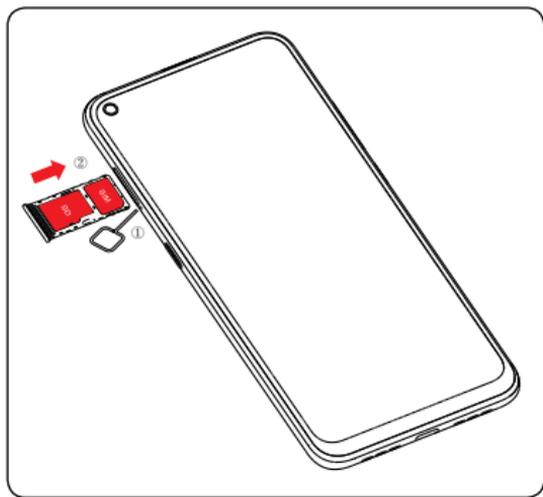
You must insert your SIM card to make phone calls. You do not need to power off your phone before inserting or removing the SIM card as this phone supports hot swap.
