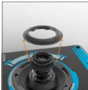
3. Remove Seal Ring
