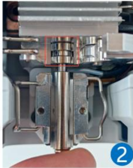
Correct demonstration (nozzle aligned with heat sink)
