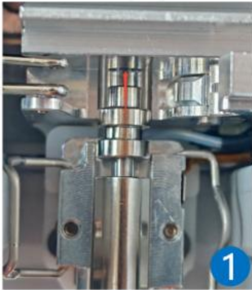
Incorrect example (nozzle not aligned with heat sink)
