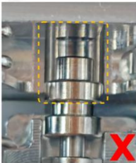
Improper installation may result in the nozzle scraping the hot bed plate, leveling errors, or other problems.
