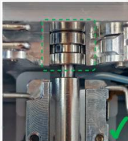
Correct demonstration (nozzle aligned with heat sink)
