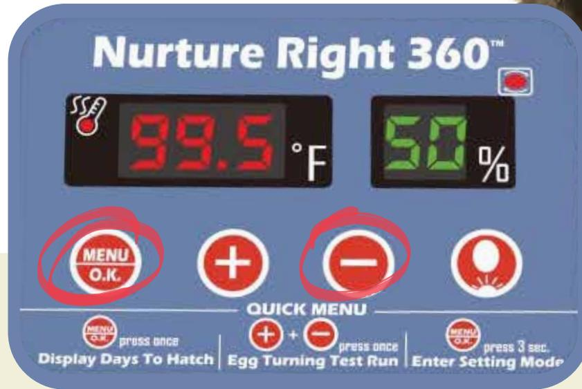
PRESS AND HOLD THE "MENU" AND "-" BUTTONS SIMULTANEOUSLY FOR AROUND 5 SECONDS. THE INCUBATOR WILL BEEP, AND THE DISPLAY WILL BLINK ONE TIME, INDICATING THAT THE INCUBATOR HAS SUCCESSFULLY BEEN RESET.
