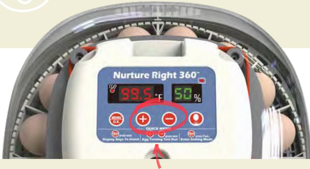
THE EGG TURNER CAN BE TESTED BY PRESSING THE "+" AND "-" BUTTONS AT THE SAME TIME!
