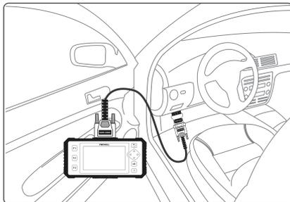
1. Locate the data link connector(DLC) under the dash on the driver side of the vehicle.
