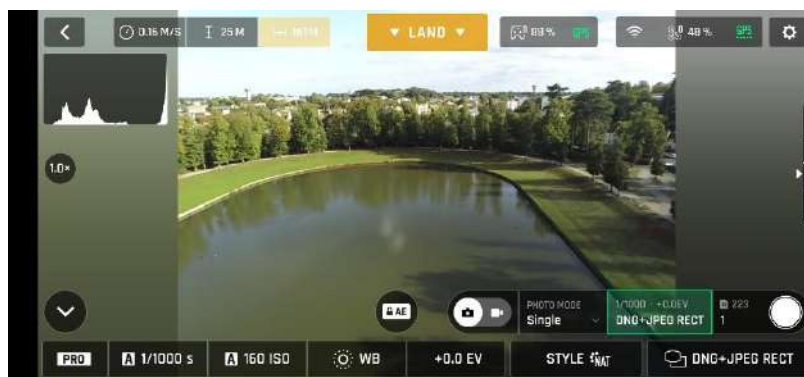
Android photo formats: DNG+JPEG RECT (zoom is unlocked, stream image is RECT)
