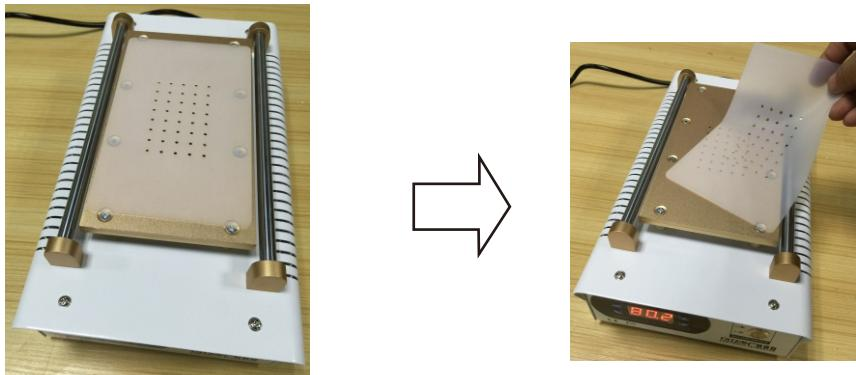
Please plug on and power on, adjust the temperature into a suitable one, the temperature we suggest is 80°C, the screen separator will damage your LCD screen if it is too high.
