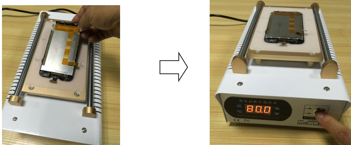
Separating the separating rods, Pull around.
