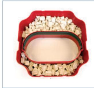
Leave enough space at the top—no nodes should be protruding from the upper edges of the baskets. **To avoid problems when stacking the baskets, there should be a minimum 5mm between the basket edge and G-nodes.**
