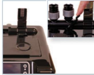
Open the cartridge lid. The silver AQUASTOP valve lever must be completely up and the black AQUASTOP release lever must be completely pushed down in order to open the lid.
