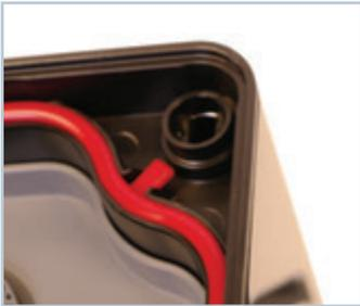
Align the red silicone seal into the black groove located around the interior rim of the canister. Run your finger all the way around the gasket to make sure it is seated properly.
