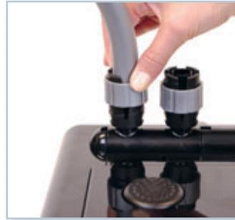
The intake hose will connect to left side of the AQUASTOP valve (down arrow). Push one end of the hose all the way onto the barbed adaptor, turn the nut counter-clockwise as tightly as possible without forcing it.
