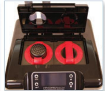
12. Align the cartridge assembly of the cartridge so the notch at the back right of the cartridge head matches the key on the motor head, and then turn the top knob clockwise to lock the cartridge into place.
