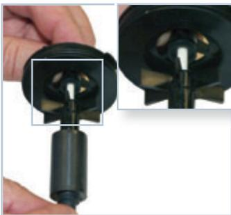
Put the ceramic shaft back into the magnet. Place the shaft back into the centre part of the cover, gently turning and pressing the rubber bushing until the ceramic shaft is all the way into the top rubber bushing.
