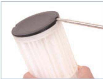
9. Debris is collected on the inside of the filter so the bottom plate needs to be removed in order to do a thorough cleaning. To remove the bottom plate, carefully insert a flathead screwdriver between the plate head and cartridge. Twist slightly and the bottom lid should come off easily. Do not force anything.
