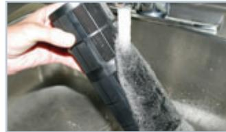
After rinsing it thoroughly with tap water, place the cartridge back into the bottom cup making sure it's properly aligned
