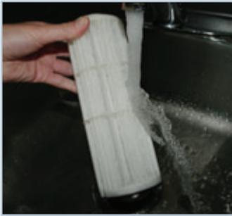
Rinse the inside and outside of the cartridge with fresh water to remove any impurities. Note that debris is collected on the interior of the cartridge.
