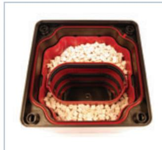
Place baskets back into the canister, carefully aligning large grooves on the baskets with the edges inside the canister.
