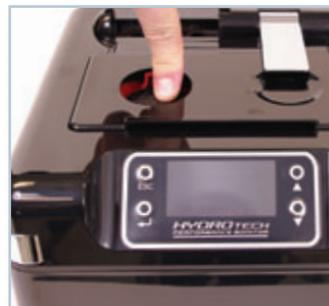
14. If no water starts circulating, push the priming button down vigorously several times. This should evacuate any trapped air and restart the water flow.
