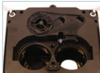
Locate the impeller cover. To remove the impeller cover, twist it counter-clockwise. Just before it releases, there will be some resistance, but keep turning the impeller cover gently until it releases upwards.
