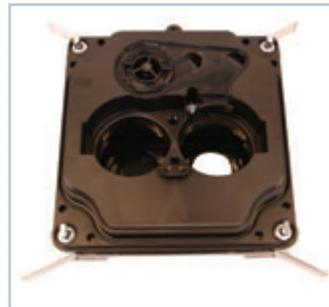
5. Open the 4 silver metal lid fasteners located on each corner of the filter. Take off the filter head, and carefully set it aside so not to damage the sensors on the underside of the lid.
