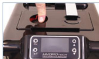
19. If no water starts circulating, push the priming button down vigorously several times. This should evacuate any trapped air and restart the water flow.
