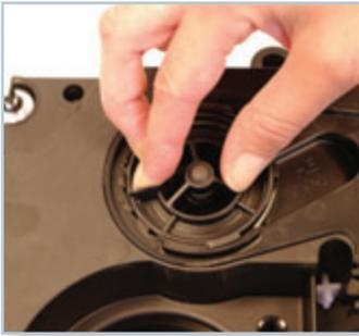
2. Locate the impeller cover. To remove the impeller cover, twist it counter-clockwise with the thumb and index finger pressed up against the tabs. Just before it releases, there will be some resistance, but keep turning the impeller cover gently until it releases upwards.
