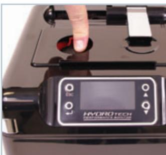
14. If no water starts to fill the filter, push the priming button down vigorously several times. This should evacuate any trapped air and restart the water flow.
