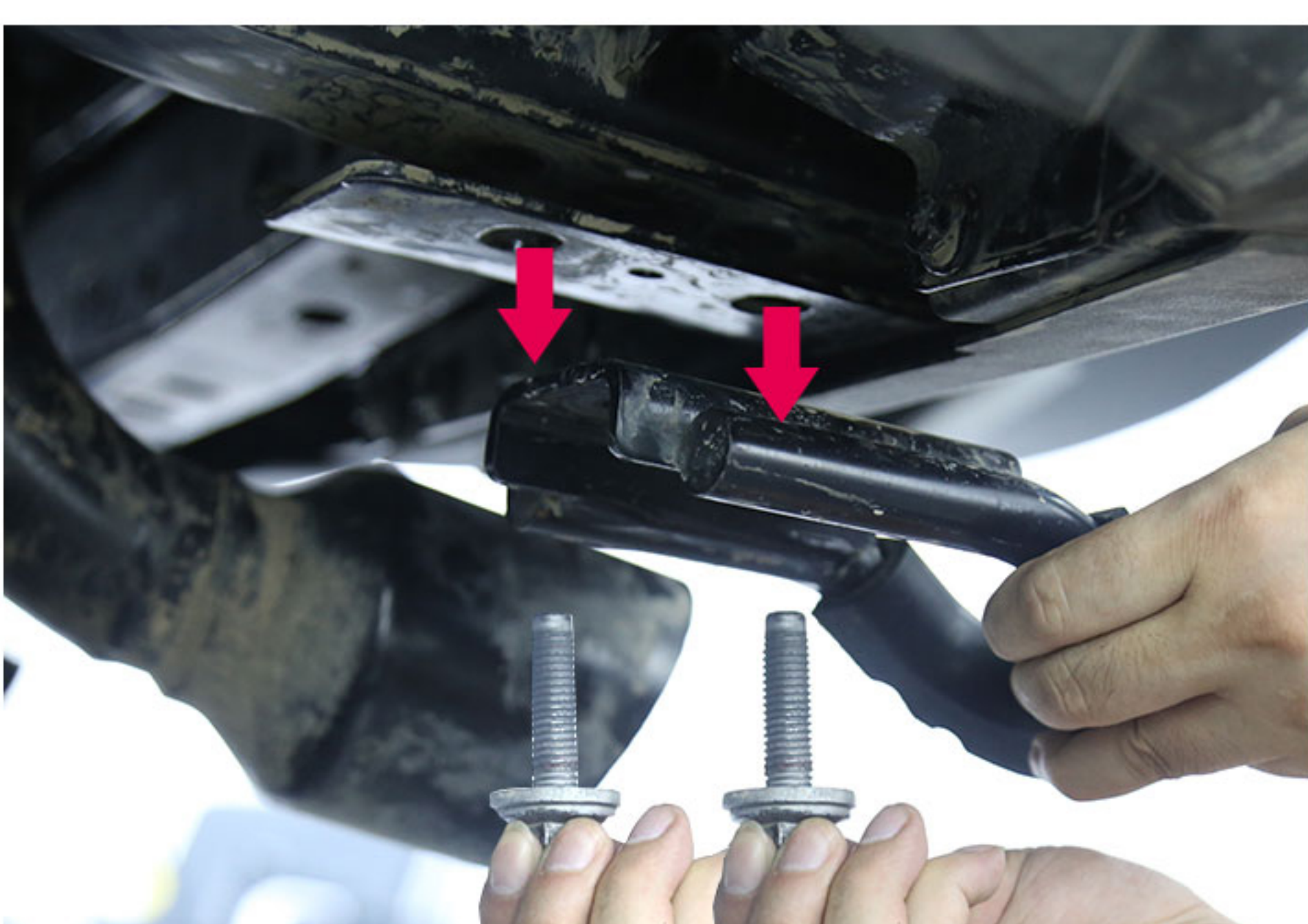
13.Detach the factory hitch tow screws.
