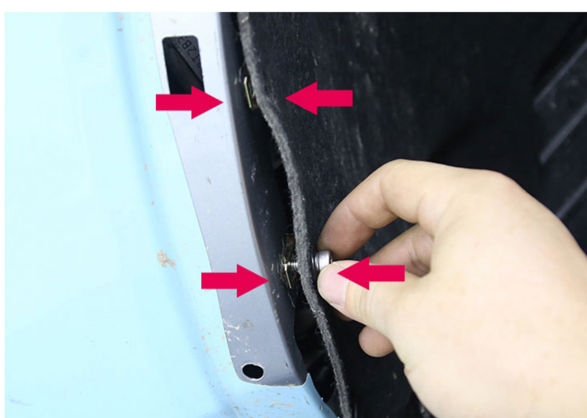
8. After the snap nut is installed, it can be screwed in normally after testing, and then remove the screw.
