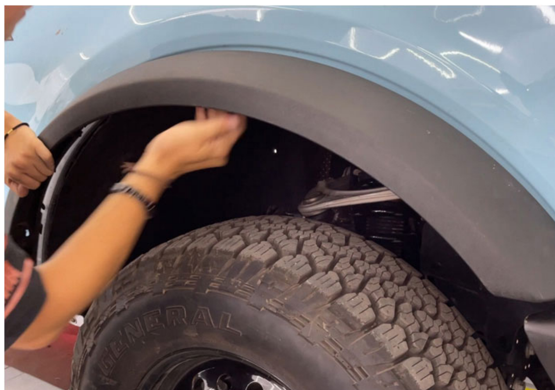
2.Detach the factory wheel fender flares.
