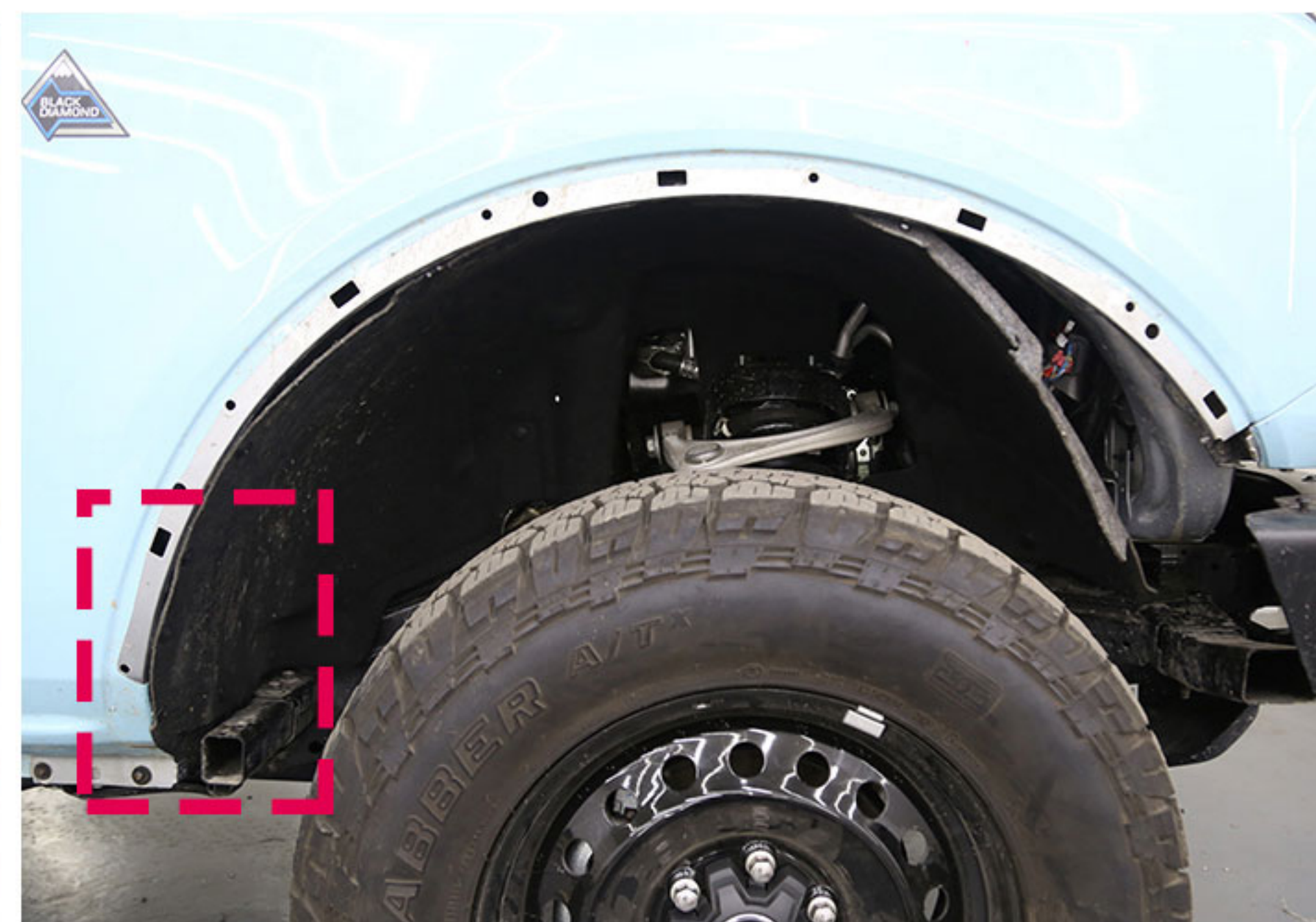
3. And then will need to install the mud flaps at this place showed in picture.
