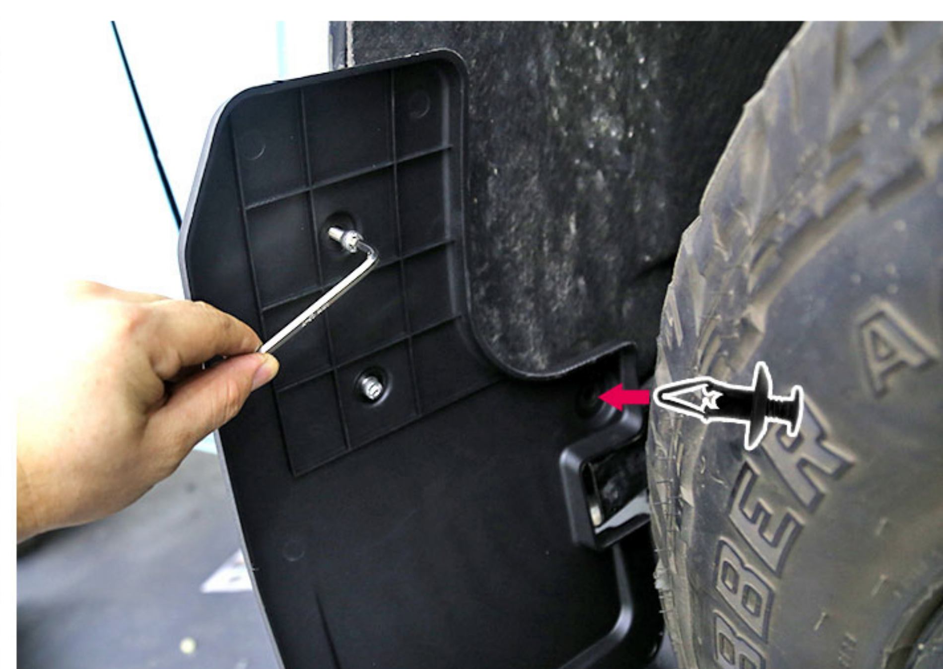
12..Install the upper fender and the original vehicle clip. If the original car clip is damaged, please use the same clip in the accessory.
