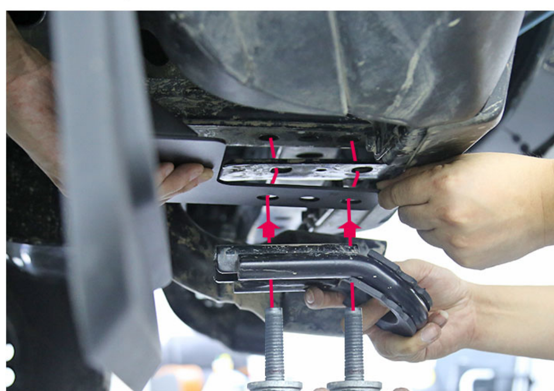
14.Install the other elements above the hitch tow by the original car holes.
