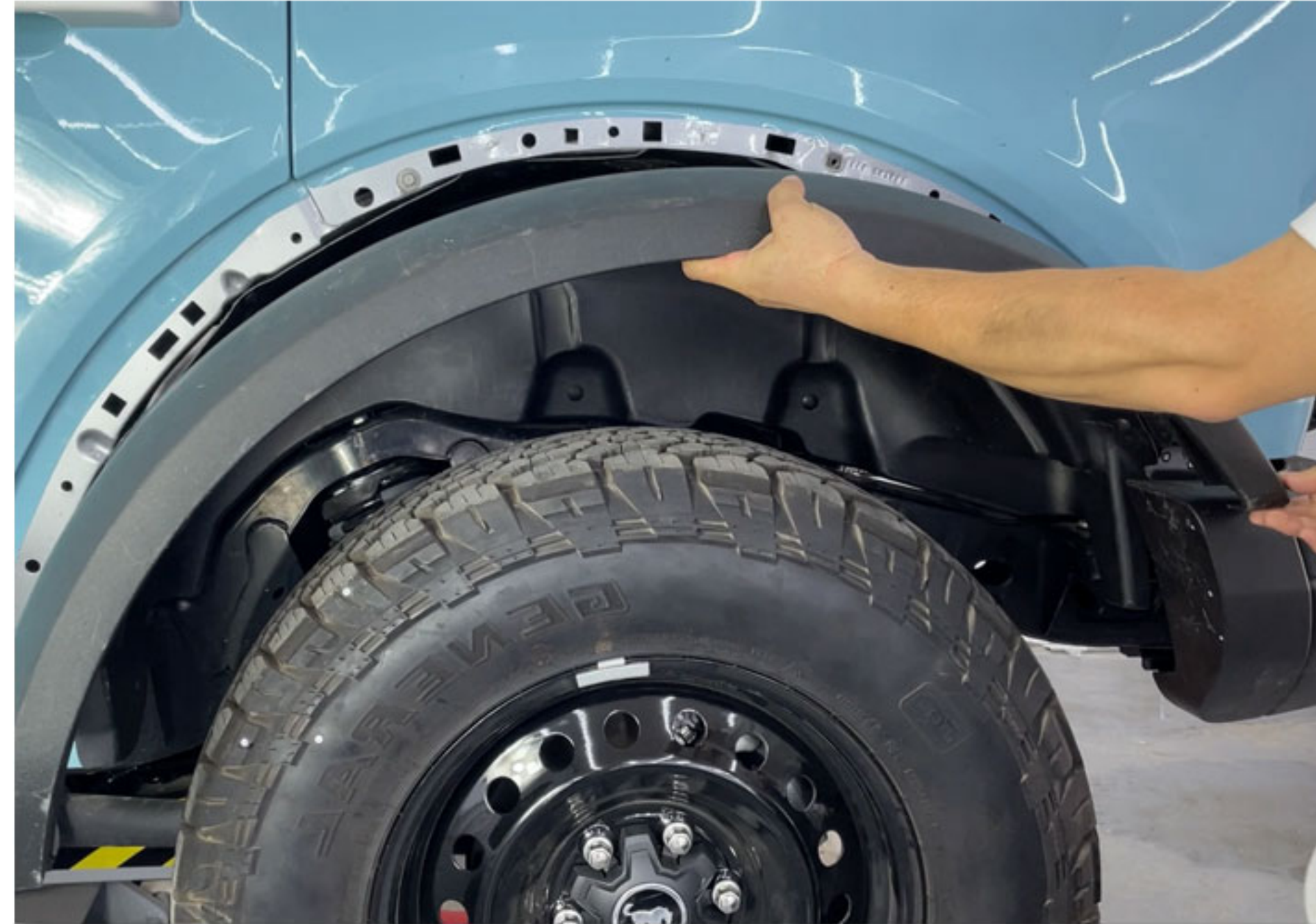
2.Detach the factory wheel fender flares.
