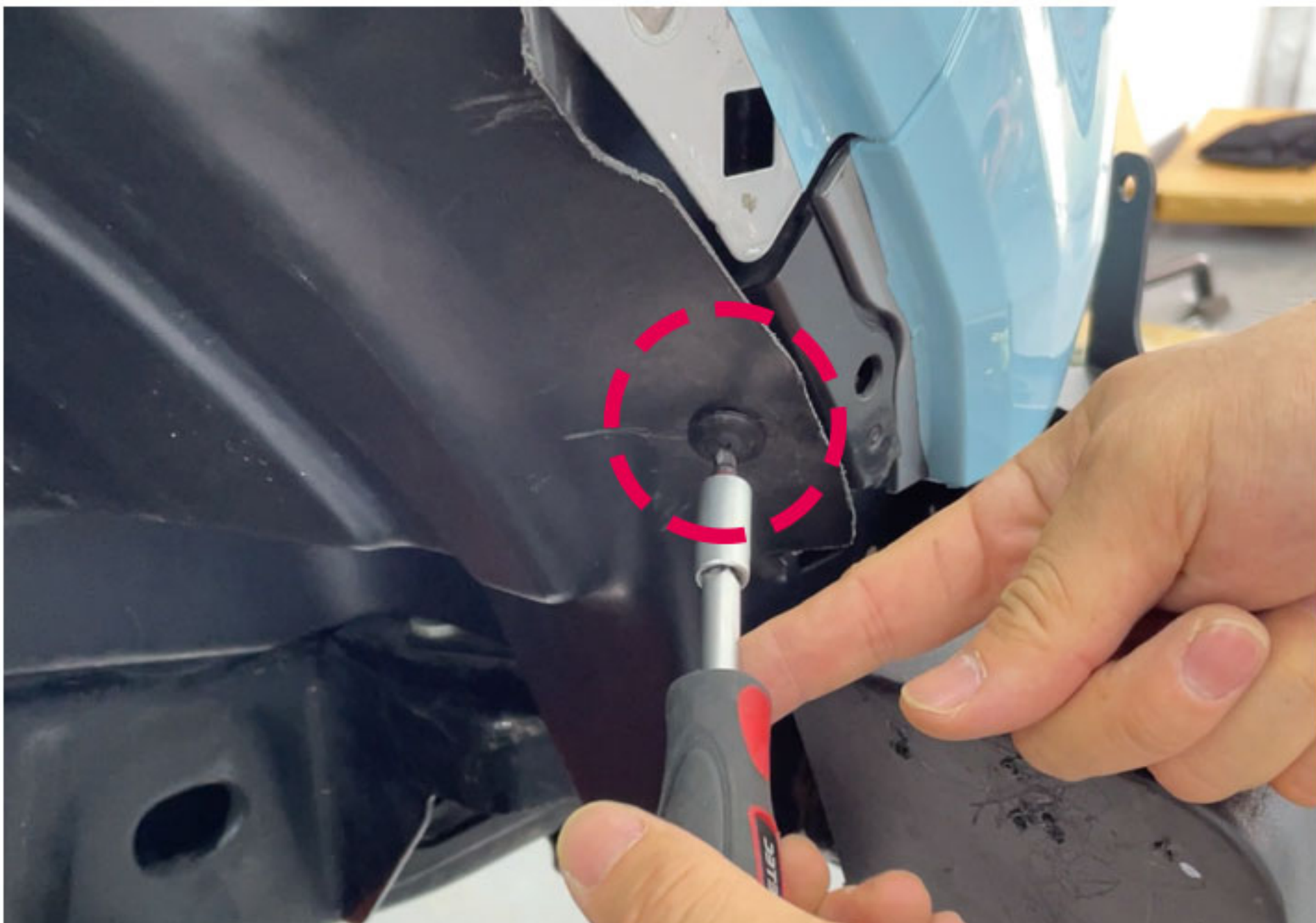
4.Detach the factory snaps from the place in circle.
