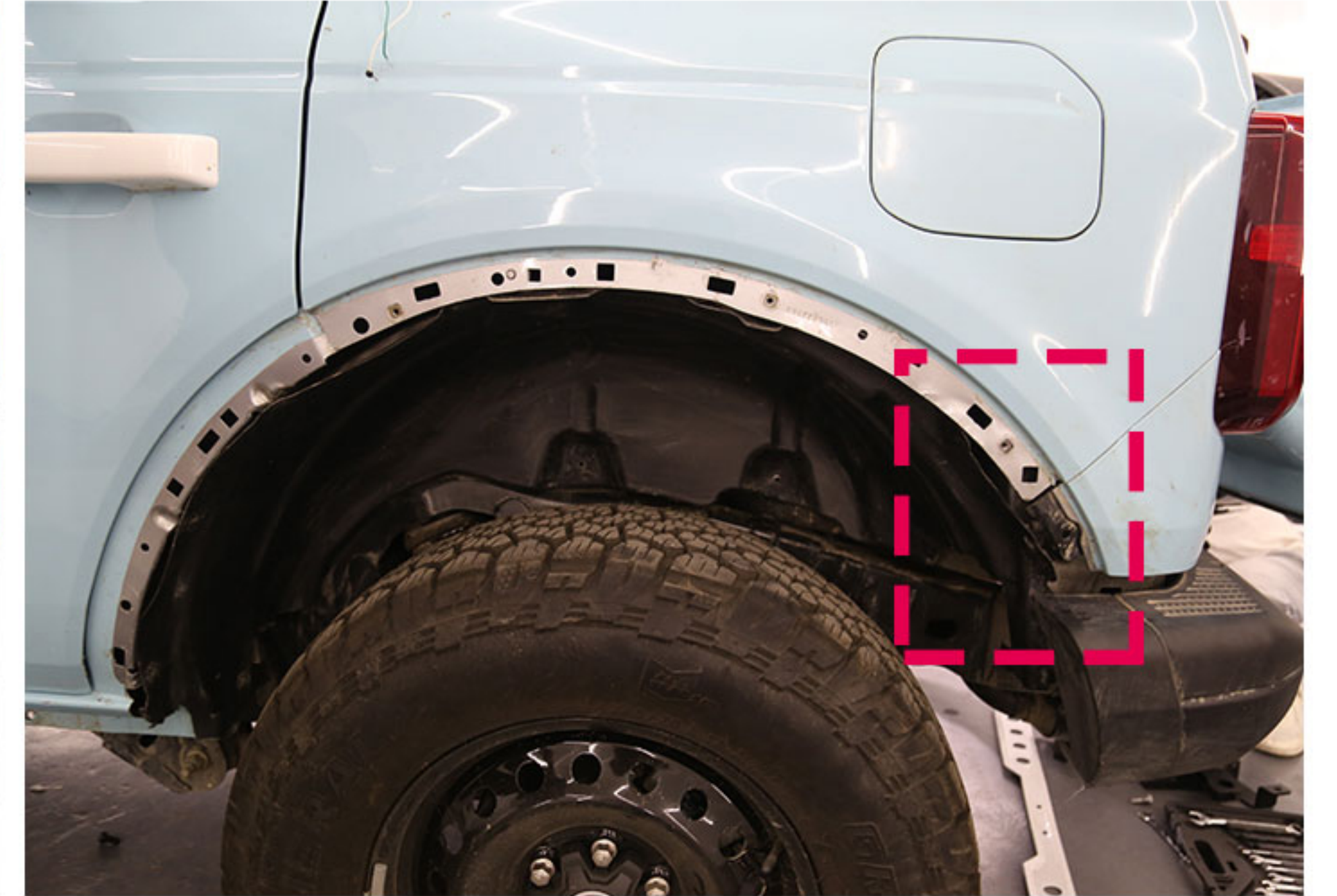
3.And then will need to install the mud flaps at this place showed in picture.
