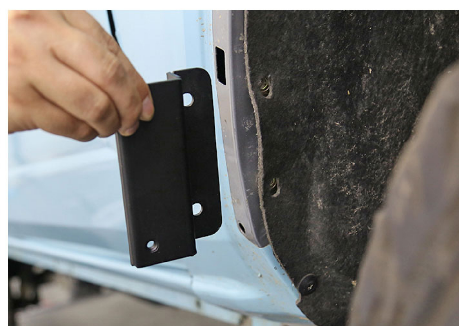
9.Install the mount as above and check the marks on the back.
