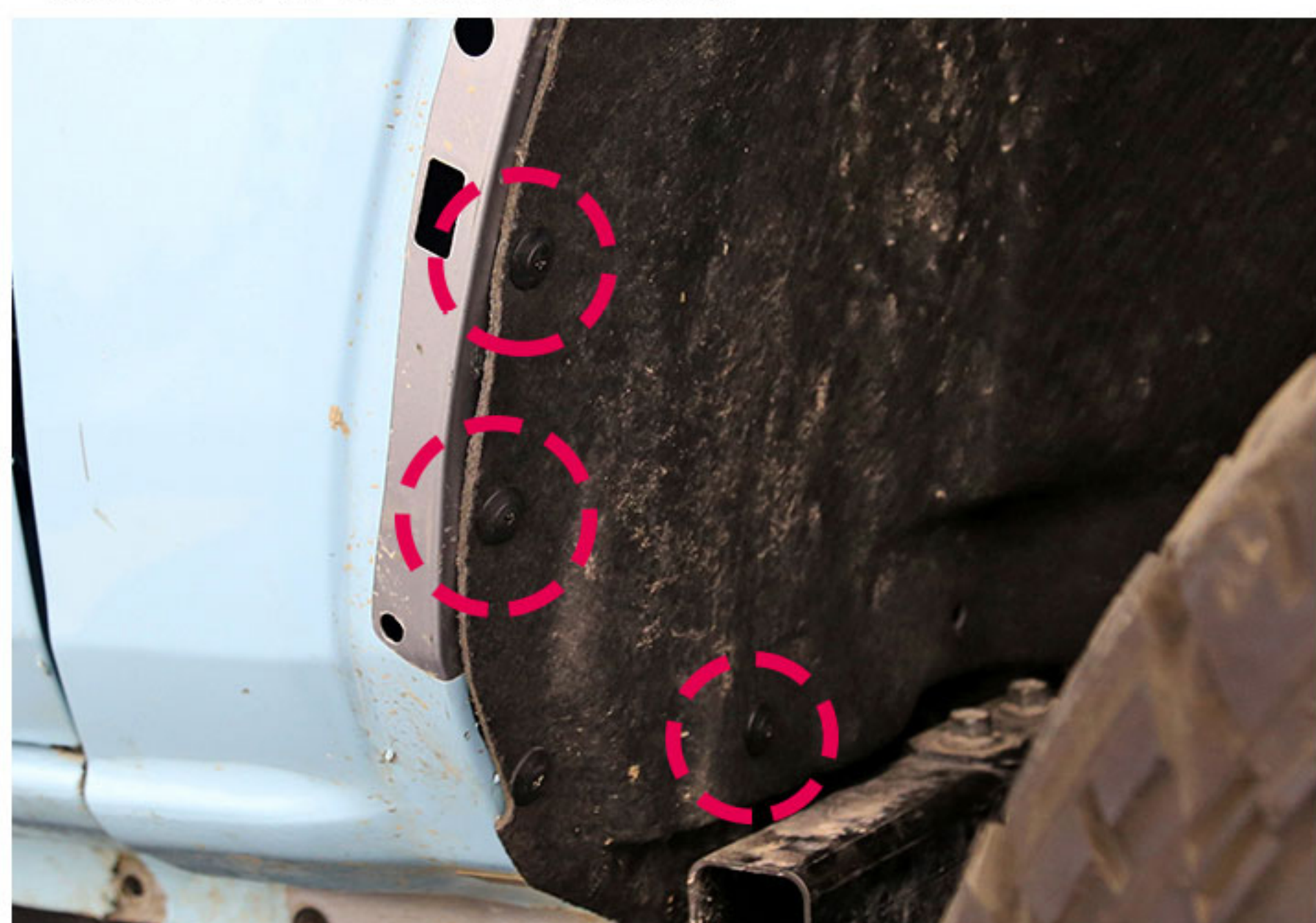
4.Detach the factory snaps from these 3 places.
