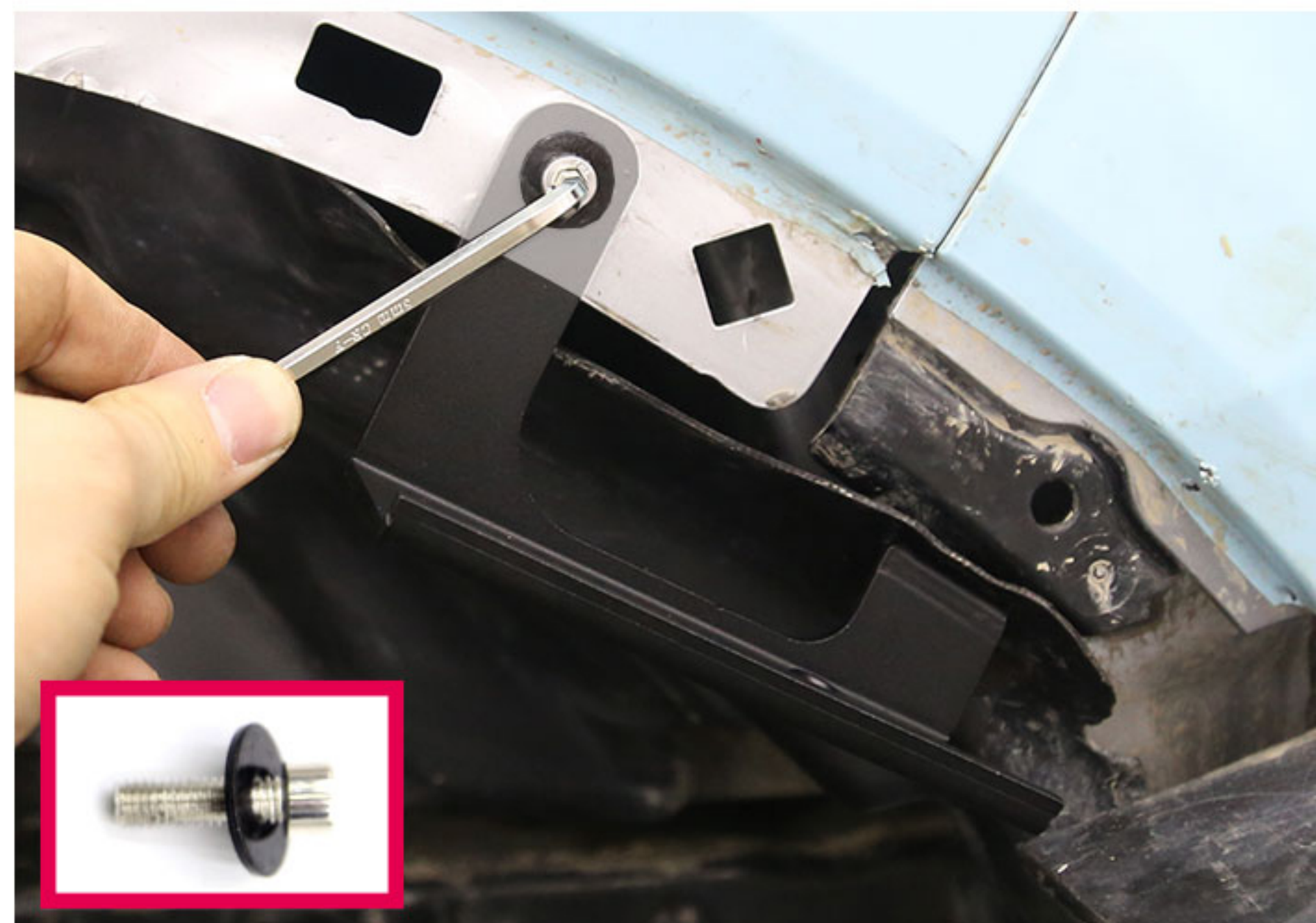
8.Put the other side of the mount in between the wheel and factory nut, and install.
