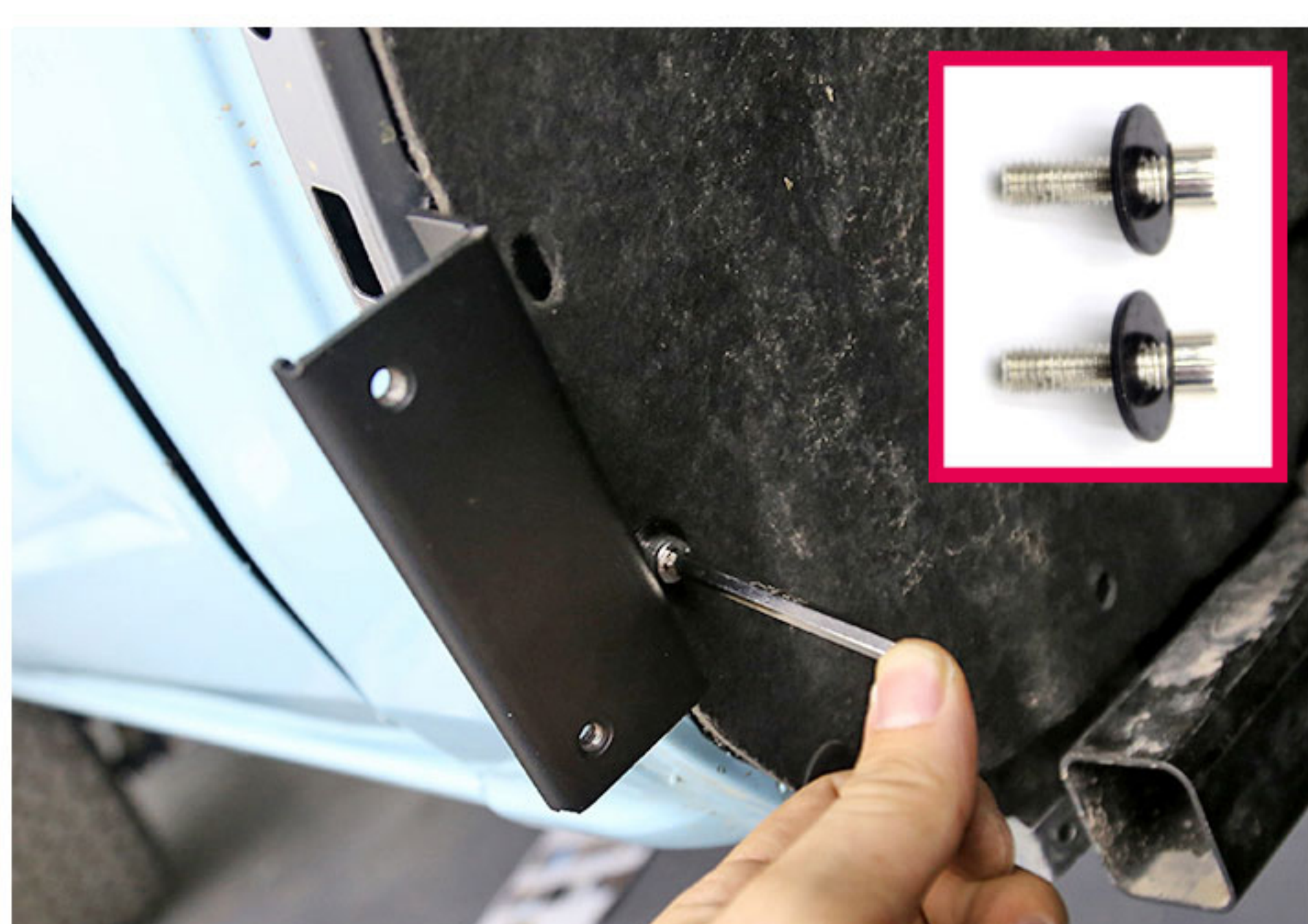
10.Screw the screws. NB: can't let snap nut move when installing.
