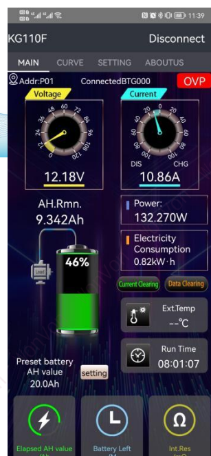
Figure 3-5-12 Over-voltage protection status
