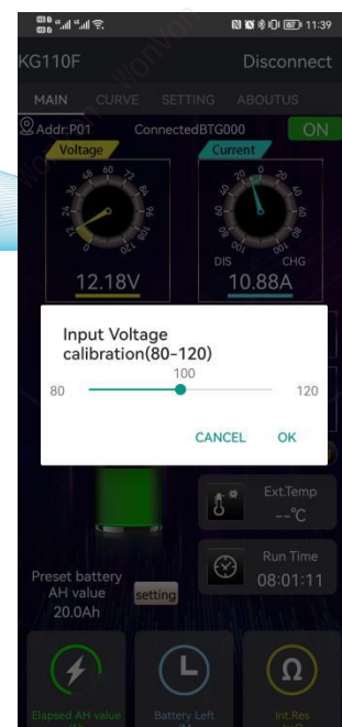
Figure 3-5-13 Input Voltage calibration
