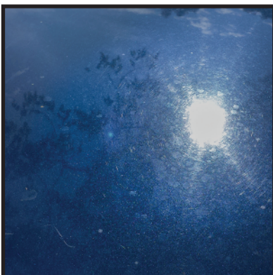
Neglected Moderate swirls, scratches, oxidation and stains
