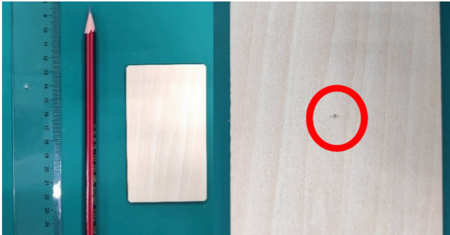
Picture 3.1 draw a center point on the engraved object
