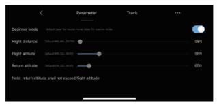
Novice mode: In this mode, the aircraft's farthest flight distance and altitude is 98ft, and the return altitude is 65ft, so that the aircraft can fly more safely within sight.
