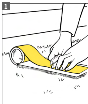
1 Cut Tape to fit opening.
