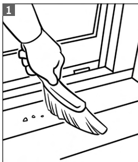
1 Clean area to be sealed.
