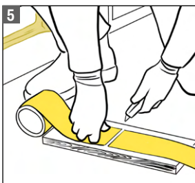
5 Cut Tape into 2-ft sections.
