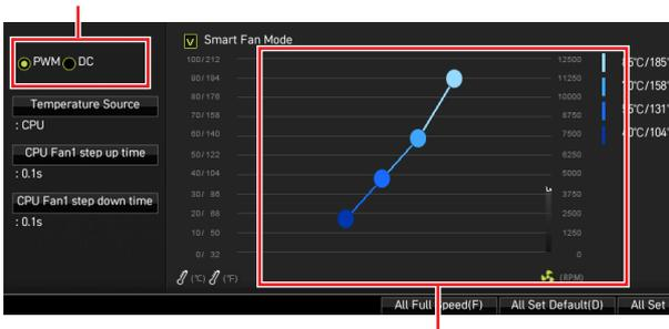
There are gradient points of the fan speed that allow you to adjust fan speed in relation to CPU temperature.
