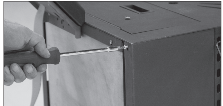
Figure 35: Remove (2) screws from rear of side panel, at the top and bottom of the panel. Remove (2) screws from the front face of the side panel, at the top and bottom of the panel.
