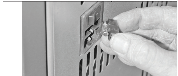
Figure 20b: Main power switch
