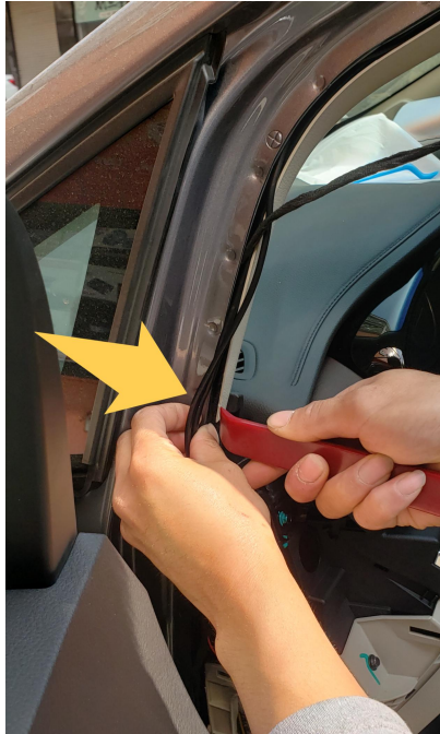
Hide the cable inside the A-pillar
