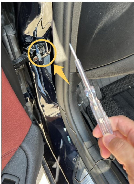
Connect circuit tester to the metal (ground)
