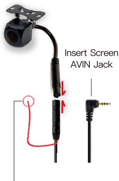
12V trigger wire, connect to the positive of the reverse light
