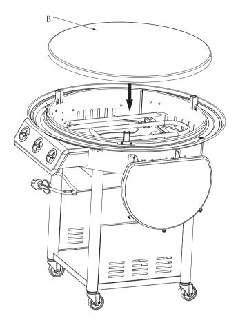
12. First, loosen screws on the underside of the lid (A). Then rotate the lid hook until it connects with the screw. Second, place the lid on top of the griddle plate.
