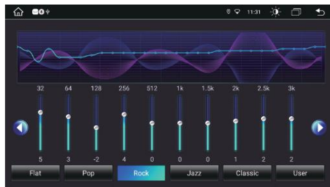
5 Equalizer: Sound effects can be set Flat, Pop, Rock, Jazz, Classic, User, Custom
