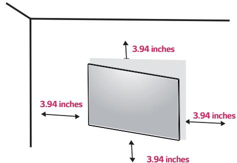
To install the monitor to a wall, attach a wall mounting bracket (optional) to the back of the monitor. Make sure that the wall mounting bracket is securely fixed to the monitor and to the wall.
