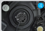
Swirl Kits into the headlight housing and secure by rotating into place
