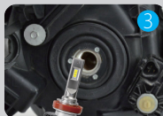
Connect the power plug, and turn on the switch to test if LED bulbs work without problem
