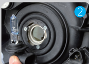
Remove the original bulb
