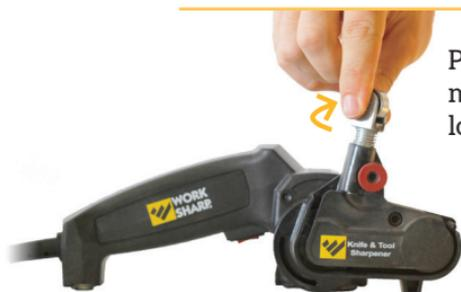
Push tensioner down and make  $\frac{1}{4}$  turn to the right to lock in place.
