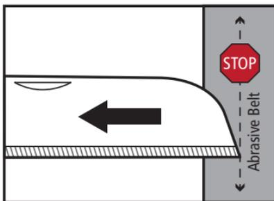
Pull straight through the guide and stop **ON** the middle of the belt. Do not lift the blade handle. Turn power off as you come to the point.
