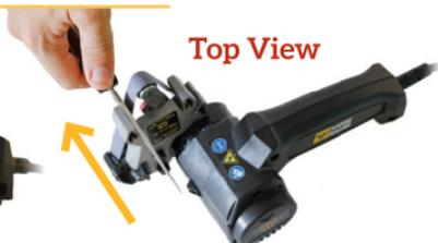
**NOTE:** Proper knife-sharpening position: blade against outer edge of guide. Place knife blade in the guide so that the side of blade is against the outside edge of the guide slot. Use only the weight of your blade as you pull through for best results.
