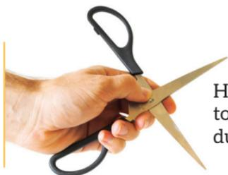
Hold scissors as shown to keep blades open during sharpening.
