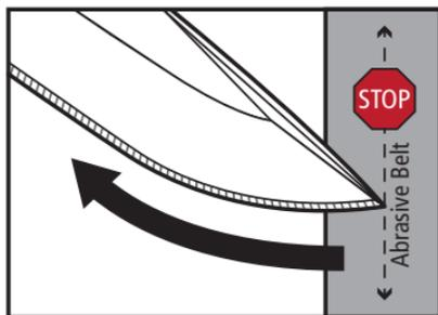
Follow the curve of the blade so the edge remains perpendicular to the belt. Turn the power off as you come to the point.
