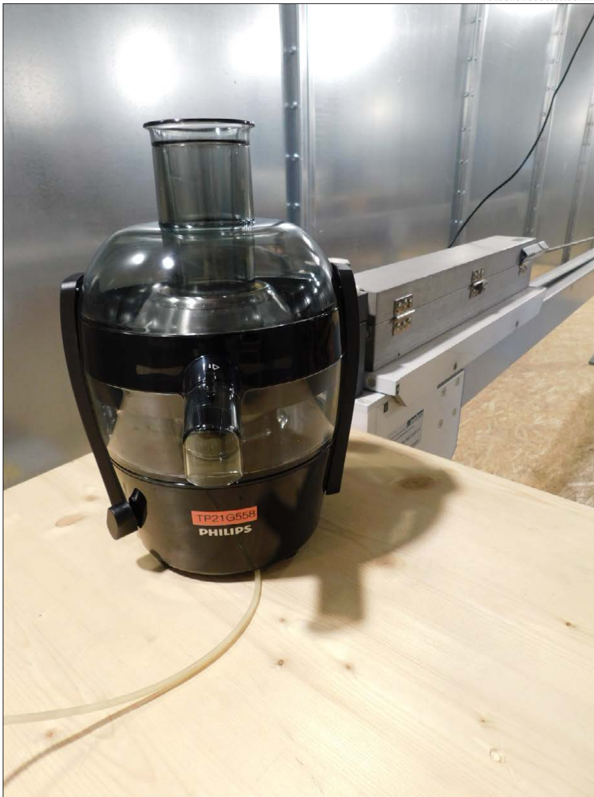
Picture 4: Test setup CISPR 14-1 disturbance power on AC power supply lines
