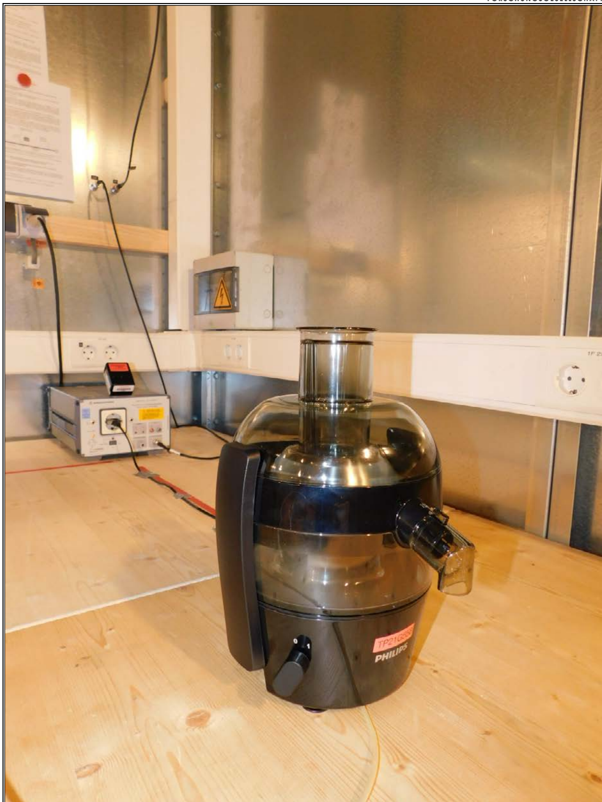
Picture 3: Test setup CISPR 14-1 disturbance voltage on AC power supply lines
