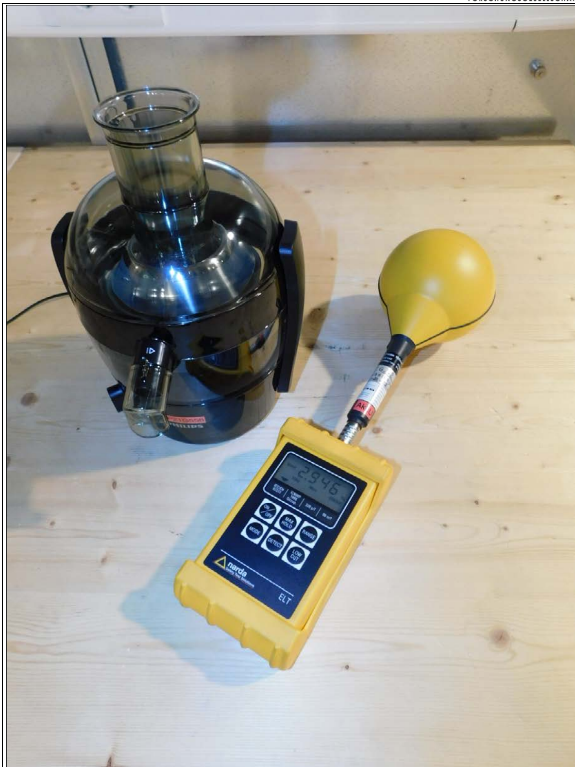
Picture 6: Test setup IEC 62233 EMF test (220 V / 60 Hz) (symbolic picture)
