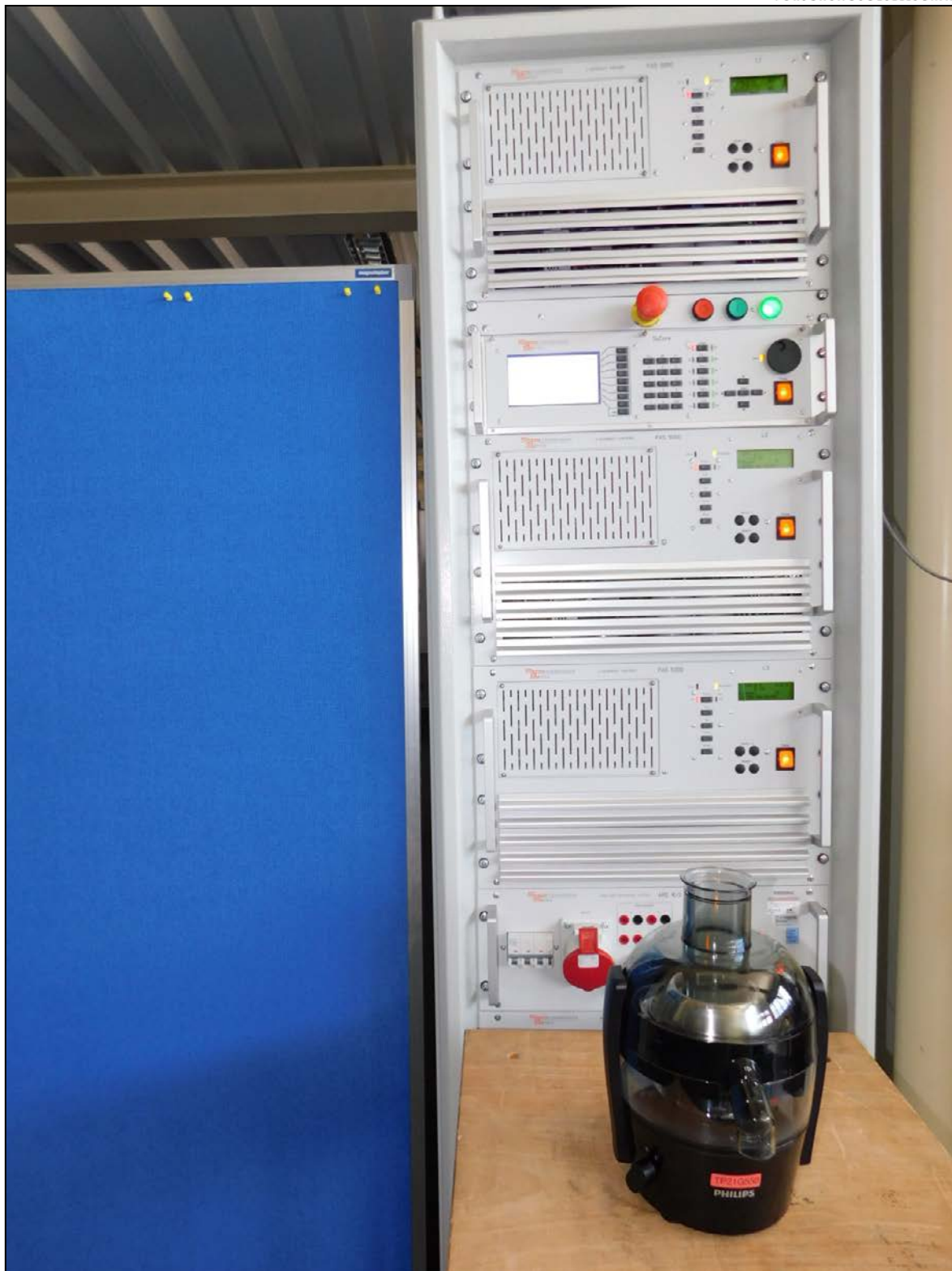
Picture 7: Test setup IEC 61000-3-2 harmonic currents / IEC 61000-3-3 flicker
