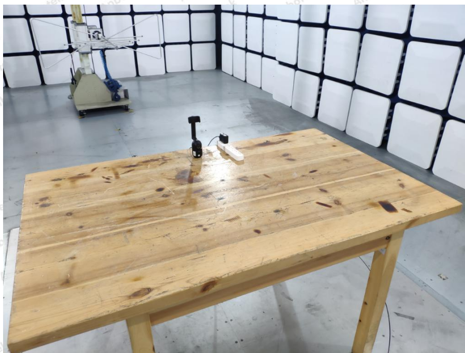
Photo of Radiated Emission Test(30~1000MHz)
