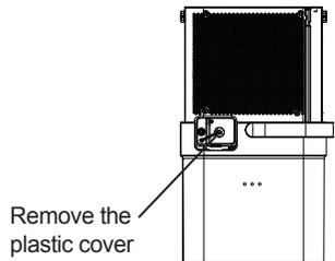
Remove the plastic cover rotating counter-clockwise
