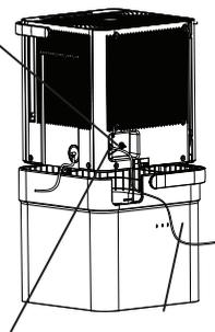
Pump drain hose outlet Pump drain hose
