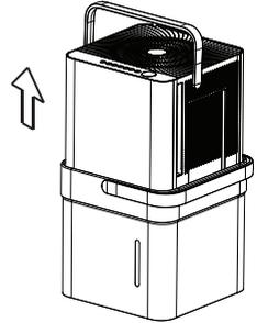
2. Lift the bucket using 2 hands and carry to drainage point.
