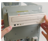
Installing an Optical Drive
