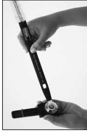
CLEANING THE PRESSURE REGULATOR
