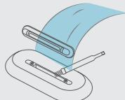
Detach the water tank from the base. Take out the water tank cover and rinse it with warm water.
