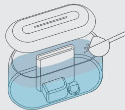
Fill the tank with a solution of bleach and water (one teaspoon of bleach for each gallon of water.). Replace the tank cover and shake around the tank.
