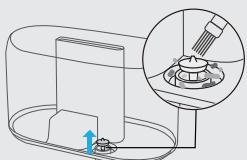
Remove any particles or hair blocking the water valve.
