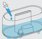
Your water tank has leakage due to prolonged use of essential oils.
