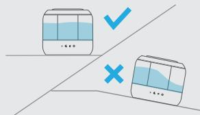
Make sure the humidifier is placed on a flat surface.
