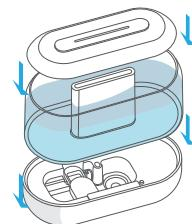
Attach the water tank to the base, replace the top cover.
