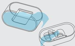
Drain any remaining water from the tank and the base.
