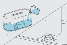
The water valve is not flat or the tank leaks water when refilling.
