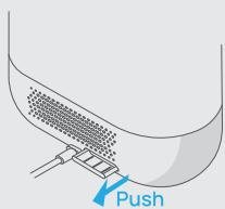
Push to open the aroma pad tray at the back of the base to pull it out.
