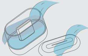
Remove the tank and detach the cover, drain any remaining solution from the tank and the base. Rinse the tank with water until the bleach smell is gone.
