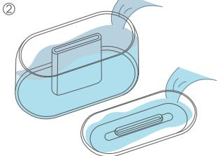
Detach the cover and water tank from the humidifier and clean thoroughly.
