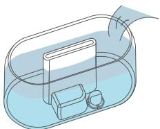
Fill the tank with room temperature water. Do not fill with hot water.
