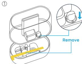
Make sure the water filter is installed correctly and the yellow label has been removed.
