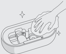
Clean the base with a soft cloth, you may use the included cleaning brush to remove excess of mineral deposit. Make sure all parts are dry before reassembling your humidifier.
