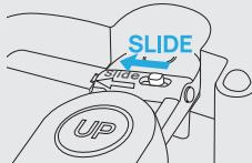
fix the left prong on the bracket, then slide the other prong to secure the float in place.
