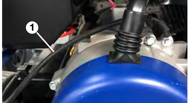
Figure 5 - Locating Negative (-) Cable
