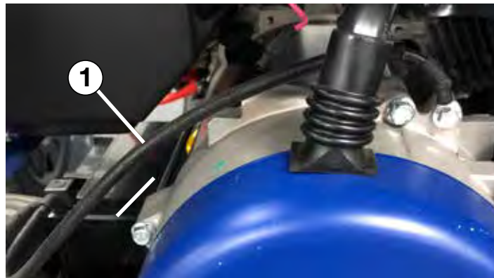
Figure 5 - Locating Negative (-) Cable
