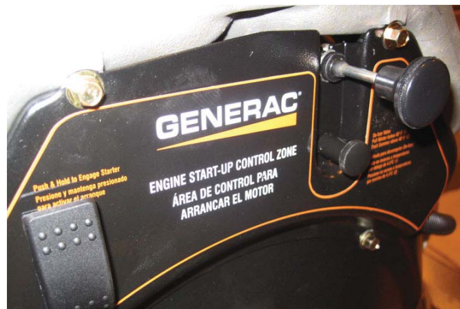
Figure 19 - Full Choke Position
