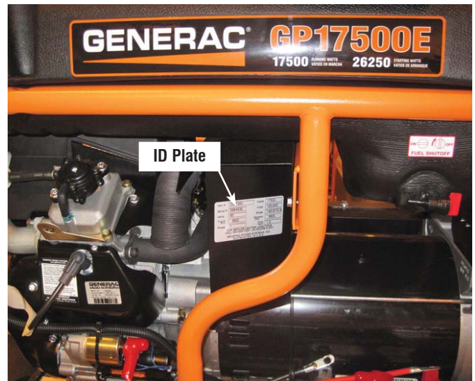
Figure 1 - Generator ID Plate
