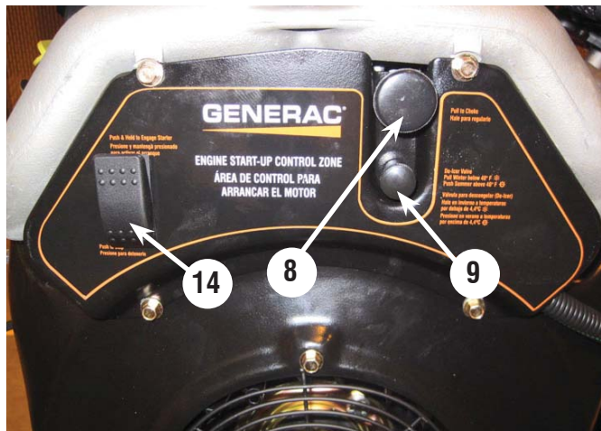
Figure 6 - Engine Control Panel
